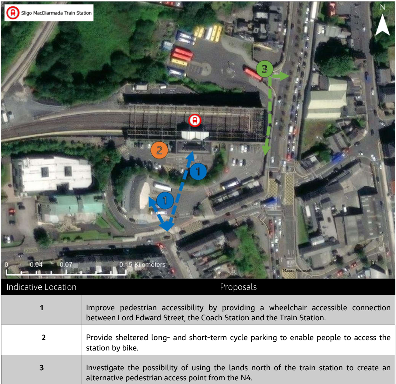
Figure 6-14: Upgrade Proposals for MacDiarmada Train Station
