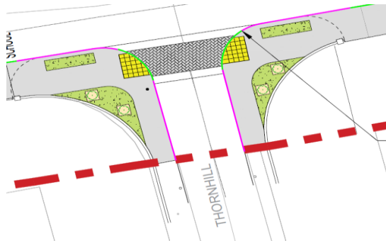
Figure 6: Indicative layout of Junction tightening measures.
