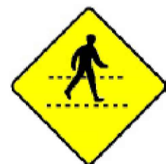
W 140A: Pedestrians Crossing
