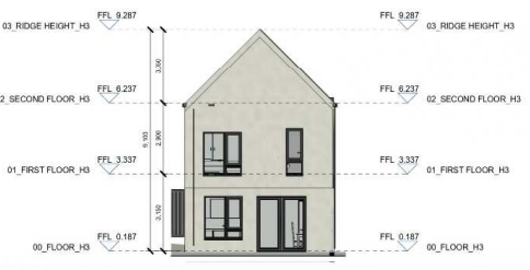
3 Bed House - Back Elevation 1:100
