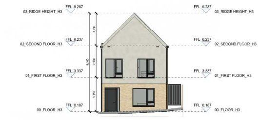
3 Bed House - Front Elevation 1:100
