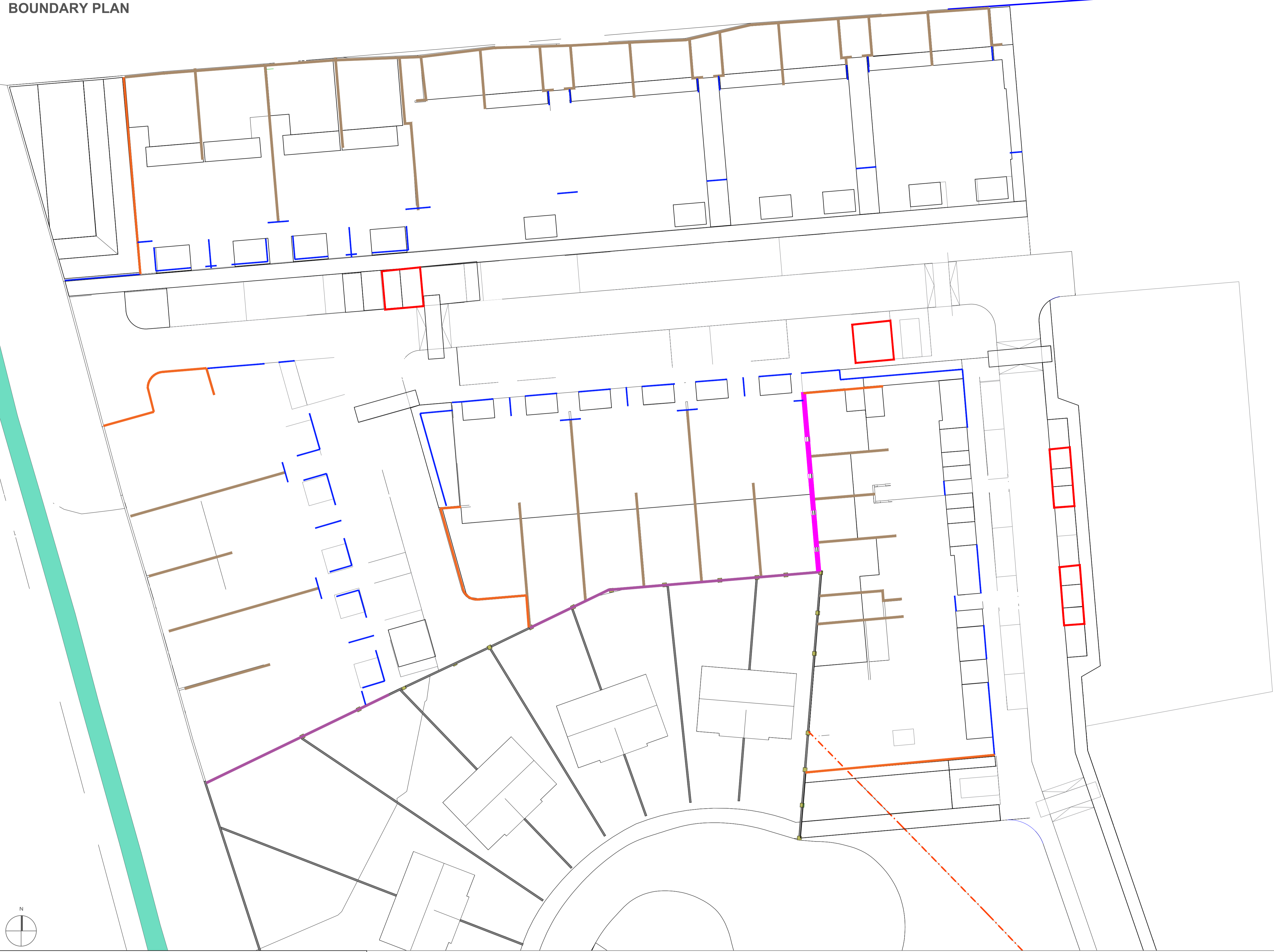
Boundary Treatment 1 Scale : 1:50 @ A1 2m high Dry Dash Wall with Concrete Piers or Similar Approved
