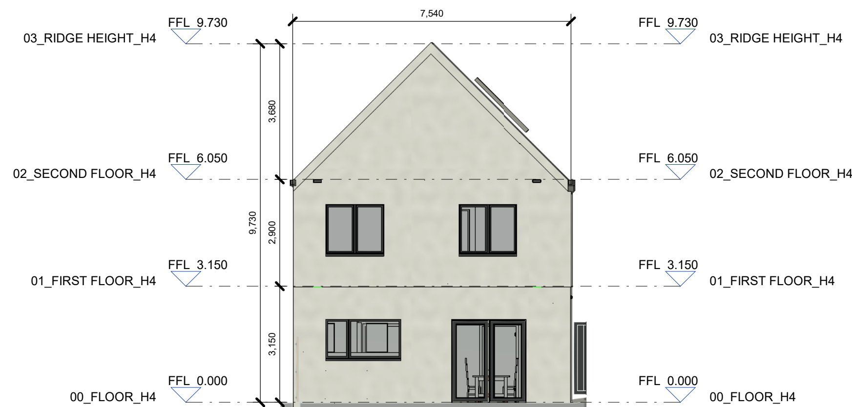
4 Bed House - Back Elevation 1 : 100
