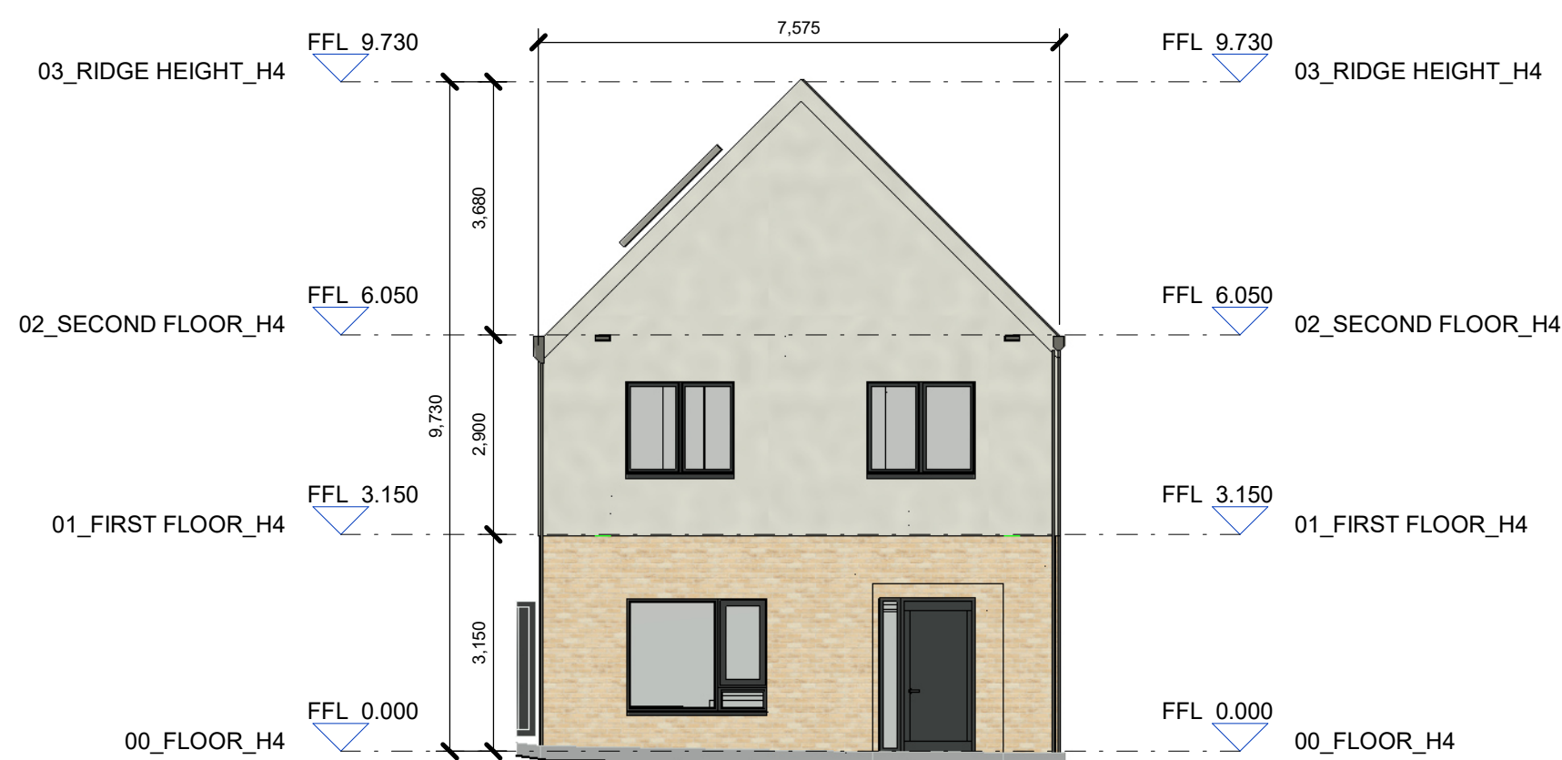
4 Bed House - Front Elevation 1 : 100
