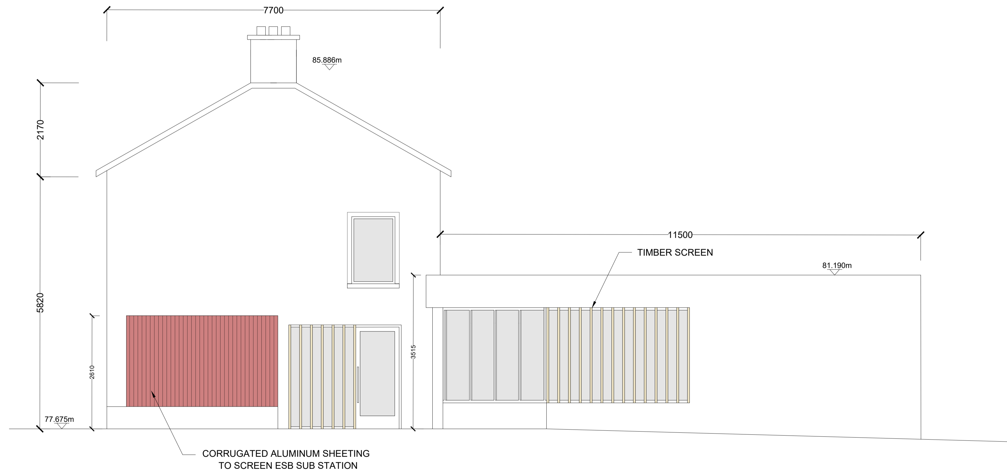
PROPOSED NORTH EAST ELEVATION SCALE 1 : 50
