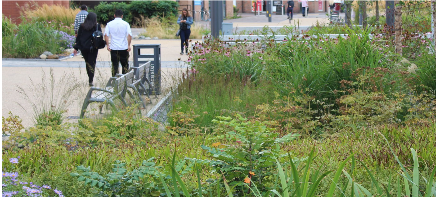
Example of planting beds using grasses and native species to accept surface water run-off at Leicester Mill Lane, UK.
